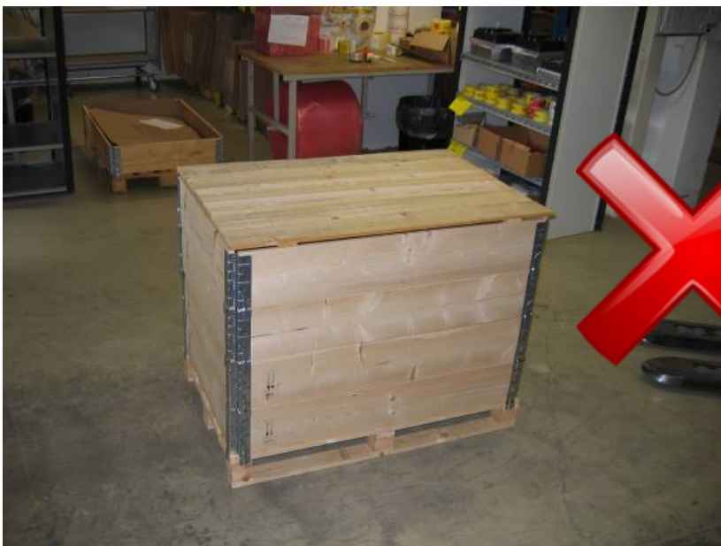
Picture 2: Not OK! 4 collars (too high), pallet lid of wood, (may leak and shed splinters onto goods).
